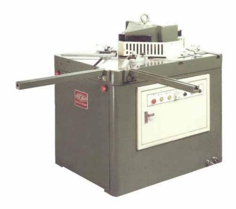
A productive, reliable, heavy-duty, hydraulic 90° corner notcher for all of your notching needs. It'll shear mild steel and stainless steel at high production speeds and is simple to operate. The operating controls are laid out for straightforward, easy access. A generous work table and sheet supports with tee slots allow the operator to maneuver large sheets.
